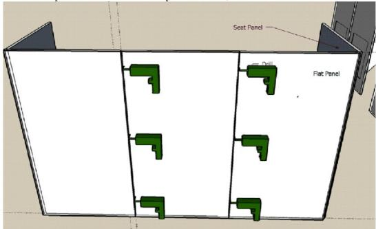
7) For the standard model (4seat) join the seat panels together parallel to each other with the same number on each side. As shown below
