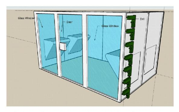
9) For two or three seat steam rooms place the single piece roof on top, when you are happy with the alignment clamp down and drill holes with 9mm bit and fix with the same technique as before, use a small number of fixings to begin E.G corners then add more till you are satisfied with the strength we recommend at least six holes along each of two sides.
