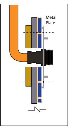
Once grouted put metal plate on wall mark holes out with pencil
