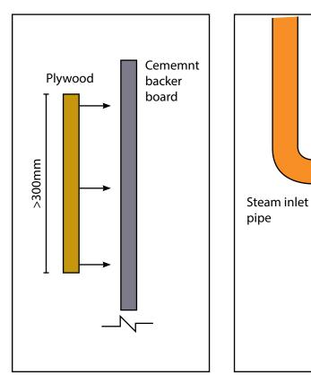
If using a cement backer board for steam room fix a square of plywood minimum 300 x 300mm behind the cement board to screw through and hold the guard in place. The cement board will not be strong enough to hold the screws on its own. Tile the room as normal and ensure the pipe with the thread is sitting forward enough so that when tiled the start of the thread will protrude 5mm past the tiles
