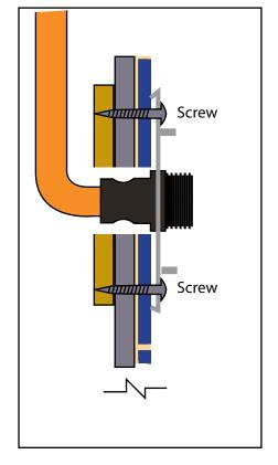
Use diamond drill to drill holes and screw through into the timber behind the backer board.
