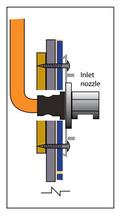
Screw the steam inlet nozzle onto the end of the steam inlet pipe Glass guard screw
