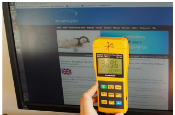
36.96mG reading in front of computer screen.
