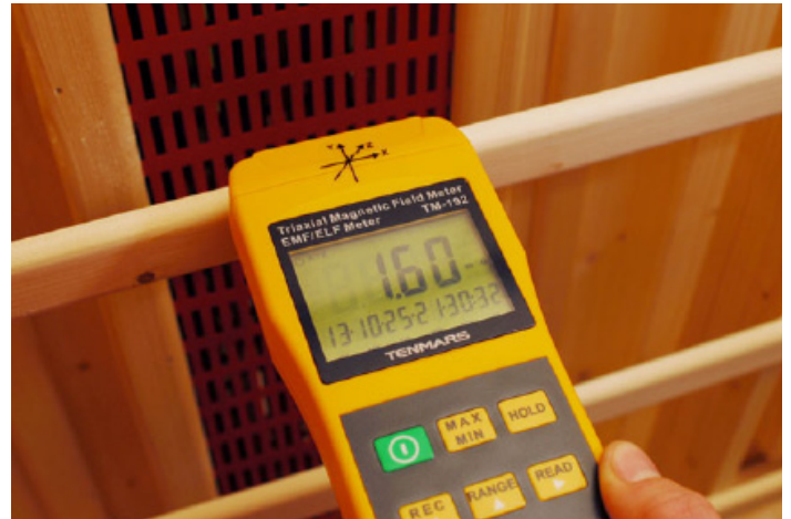
1.60mG reading at the backrest inside of Oceanic Infrared sauna
